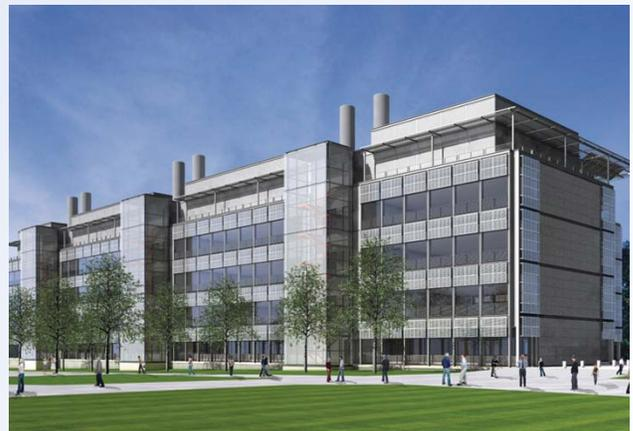
The chemistry building now under construction serves as a model for the use of aggressive energy efficiency measures to meet sustainable building goals. For example, high-performance glazing in combination with sensors for control of dimmable lighting systems will allow optimal use of ambient daylight while high-efficiency laboratory fume hoods will minimize energy loss.
